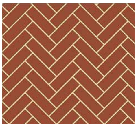
Typical Herringbourne Pattern Panel set out.
